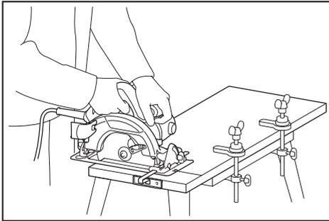
5. **Hold the power tool by insulated gripping surfaces only, when performing an operation where the cutting tool may contact hidden wiring or its own cord.** Contact with a "live" wire will also make exposed metal parts of the power tool "live" and could give the operator an electric shock.
