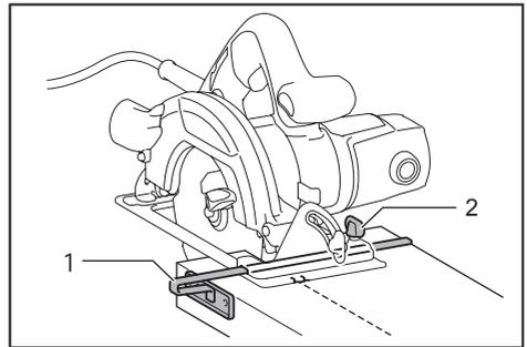
► 1. Rip fence (Guide rule) 2. Clamping screw
