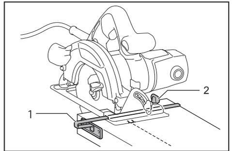
► 1. Rip fence (Guide rule) 2. Clamping screw
