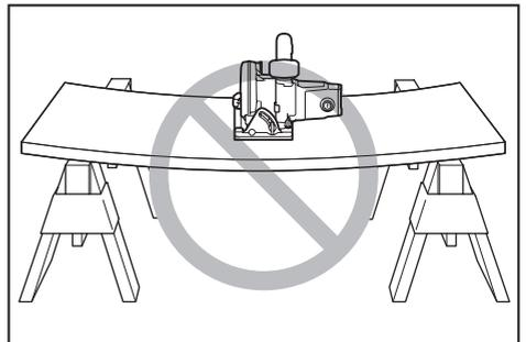
5. **Do not use dull or damaged blades.** Unsharpened or improperly set blades produce narrow kerf causing excessive friction, blade binding and kickback.
