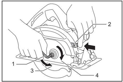
► 1. Hex wrench 2. Shaft lock 3. Loosen 4. Tighten
