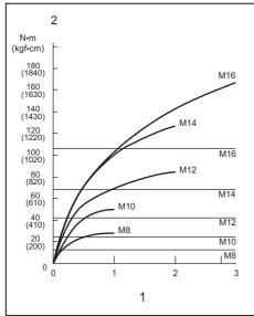
1. Fastening time (second) 2. Fastening torque
