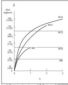
1. Fastening time (second) 2. Fastening torque ed with
